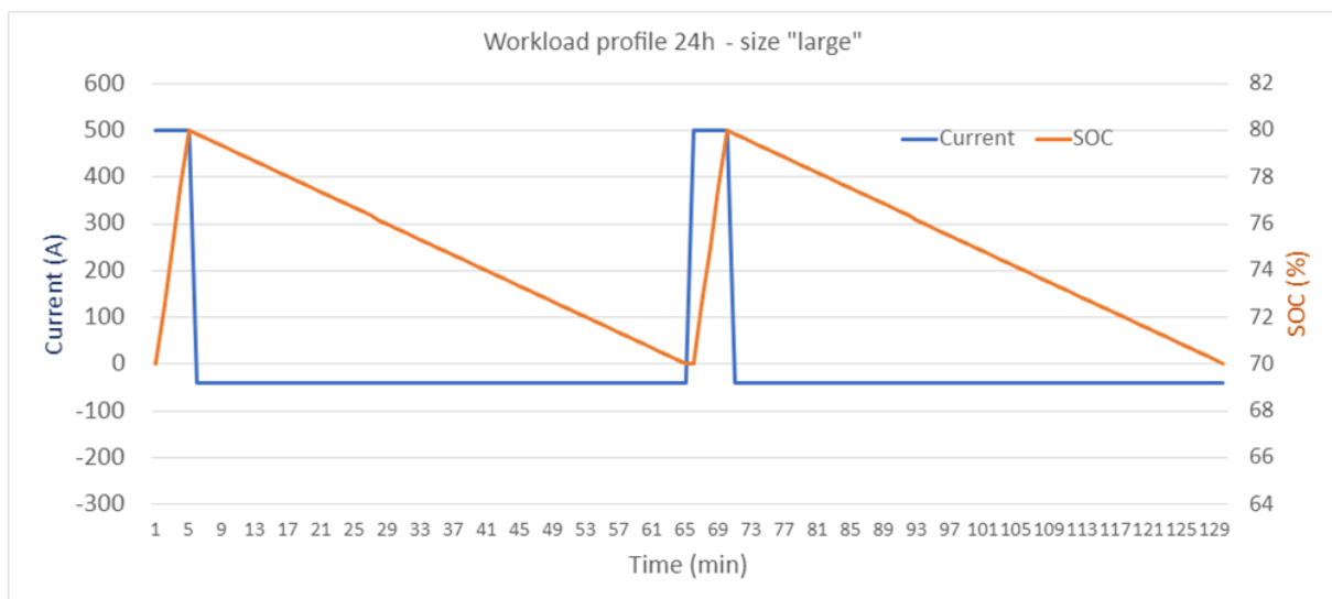
Figure 2. Exemplary Load Profile for large off-road mobile device.
