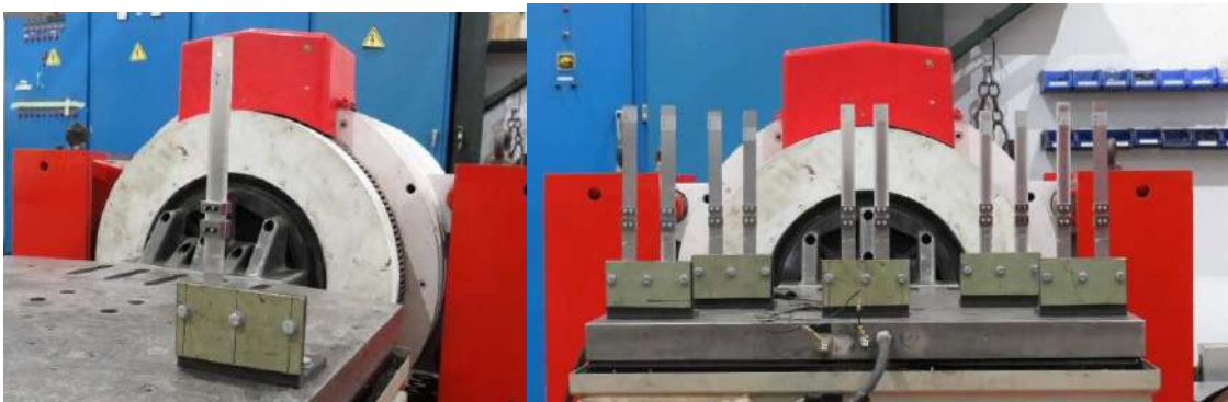
Figure 3 - SSM specimens mounted in shaker table for vibrational fatigue evaluation
